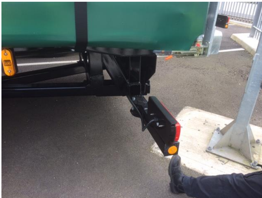
Fig No. 3 Low tail bar on semi-trailer suitable for Fork Lift 'Piggy Back'
