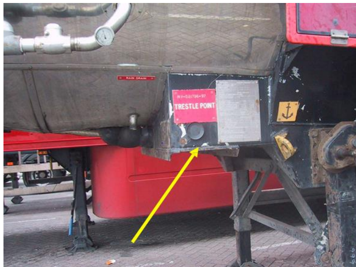
Fig No. 11 Example of a suitable trestle points on a tank unit.
