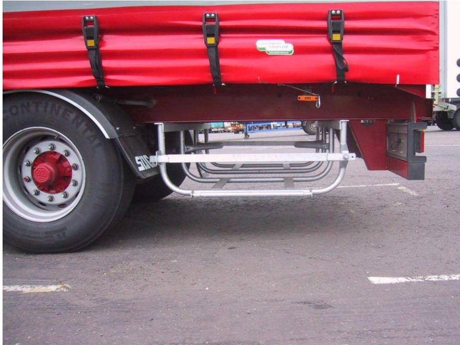
Fig No. 3 Low tail bar on semi-trailer suitable for Fork Lift 'Piggy Back'
