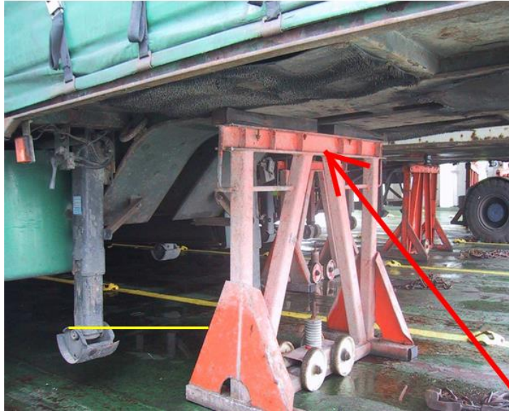
Fig No. 11 Example of a suitable trestle points on a tank unit.
