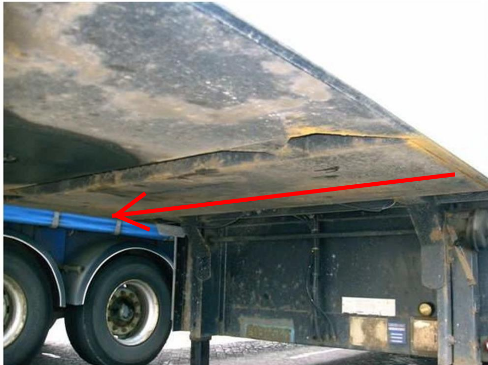
Fig No. 7 Example of the load bearing area suitable for placement of a trestle along the marked arrows.
