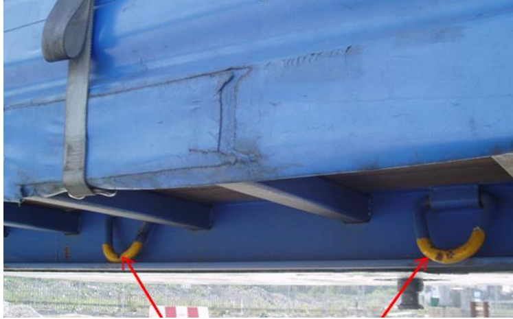
Fig No. 13 & 14 Clearly marked and well-located securing/lashing points
